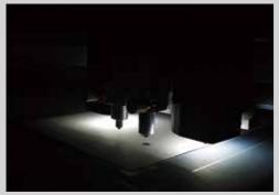
The FC-5000VC uses a high resolution camera for accurate detection of registration marks (as small as 5 mm) and can see reg marks on both colored and transparent materials. The ability to scan small reg marks saves material, thus reducing production costs.
