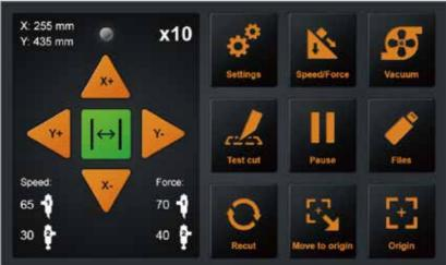
Easy toggle of vacuum suction: ON - fast/stable hold, OFF - easy replacement of next item Easy toggle of arrow key speeds for carriage control: Fast (x10) / Slow (x1) Single key press to set origin or return to origin - guarantees accurate positioning. Re-cut button to instantly repeat last job.
